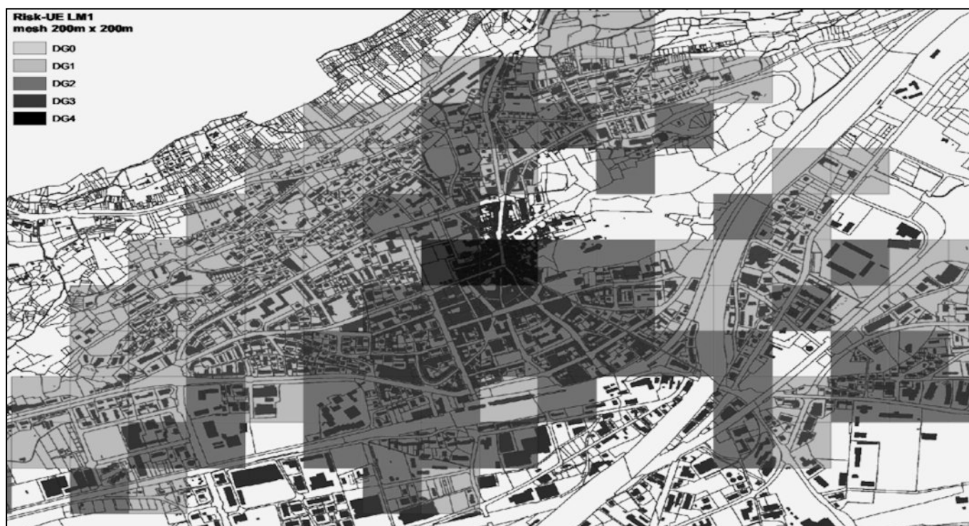
Figure 4 - Method LM1: results for the city of Sion for macroseismic intensity I_{EMS}=7.19 , with average damage grades for a mesh of 200 m x 200 m [Figure taken from: Lestuzzi et al., 2016A]
