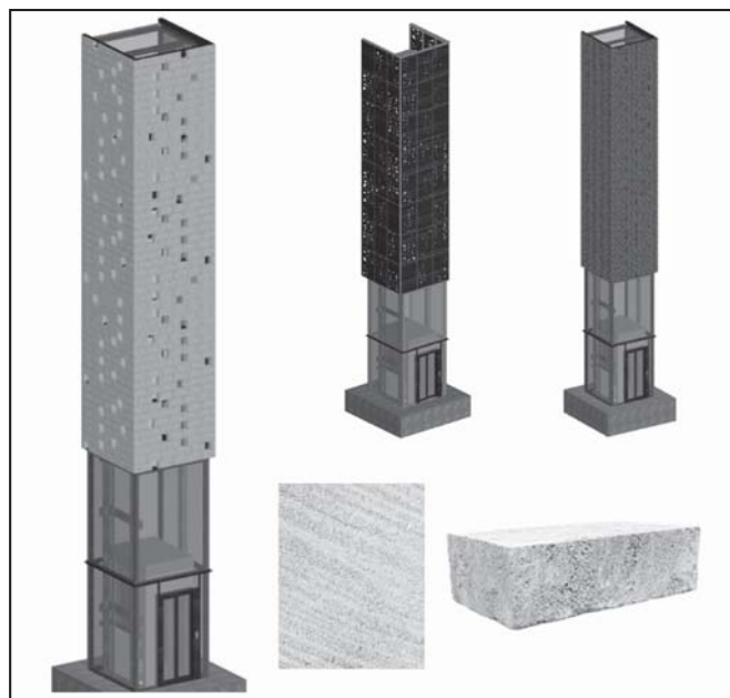
Figure 5 - The three hypotheses proposed for the cladding of the ascent hectometric systems and the chosen solution (on the left).
