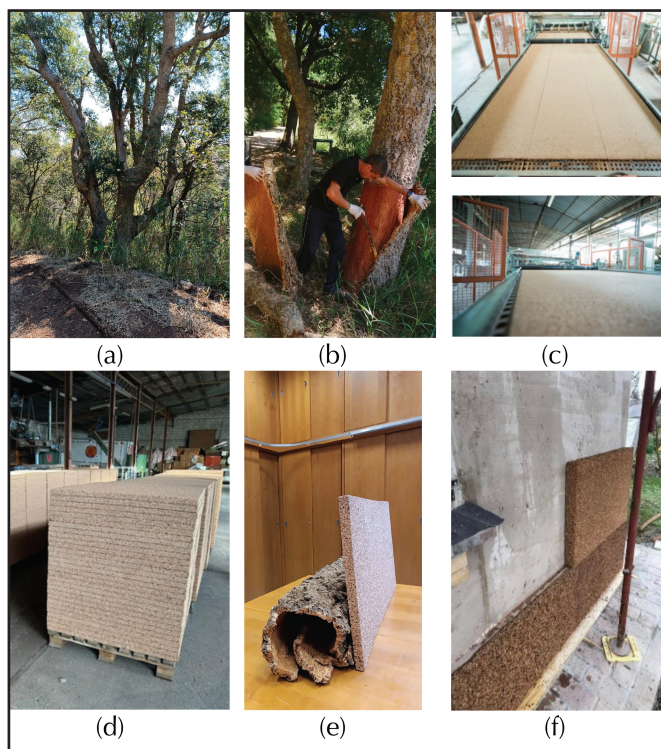
Figure 1 - Cork board production process: (a) Forests, natural origin of cork cycle; (b) Cork de-barking; (c-d) Ecological organic natural cork boards/panels production; (e) Cork: raw bark and board/panel for Green Buildings; (f) Ecological cork boards/panels make the Building: Green and Healthy. Source: Authors.
